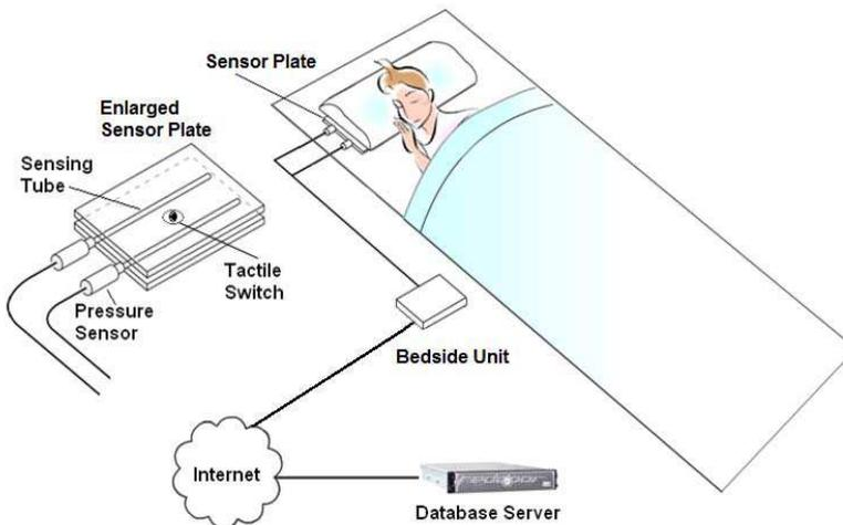
Fig. 3. Schematic illustration of the invisible monitoring of vital signs during sleep. A sensor plate is placed beneath a pillow. Signals reflecting pressure changes under the pillow are detected, digitized, and transmitted to a database server via the Internet by a bedside unit.
