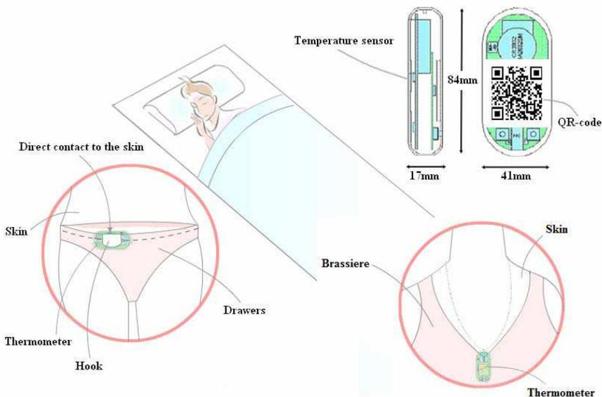
Fig. 8. A small, light wearable device (size =  $41 \times 84 \times 17$  mm<sup>3</sup>, weight = 59 g) for cutaneous temperature measurements during sleep (QOL Co. Ltd., 2008).
