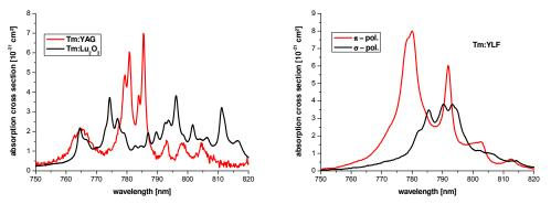
Fig. 3. Absorption cross sections of the  ${}^{3}H_{6} \rightarrow {}^{3}H_{4}$  transition for Tm:YAG, Tm:Lu<sub>2</sub>O<sub>3</sub>, (Koopmann et al. 2009b) and Tm:YLF.
