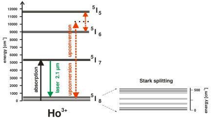
Fig. 6. Ho:YAG energy scheme with the relevant transitions for  $2.1 \,\mu m$  laser operation
