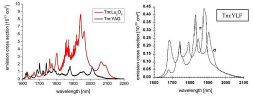
Fig. 4. Left side: Emission cross sections of Tm:YAG and Tm:Lu<sub>2</sub>O<sub>3</sub> for the transitions from the  ${}^{3}F_{4}$  manifold to the ground state (Koopmann et al., 2009b). Right side: Emission cross sections for  $\pi$  and  $\sigma$  polarisation of Tm:YLF (Budni et al., 2000).
