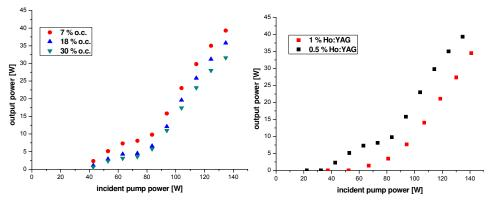
Fig. 10. Left side: Characteristic curves of a 0.5 % doped Ho:YAG rod with a length of 62mm for different output couplings (o.c.). Rigth side: Comparison of the output power for the 0.5 % and the 1 % doped crystal using 7 % o.c..
