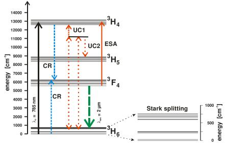
Fig. 2. Tm:YAG energy scheme with the relevant transitions for the 2  $\mu m$  laser emission and the Stark splitting of the ground state
