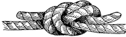
FIG. 19.—Ordinary knot (finished).
