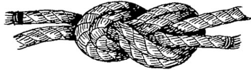
FIG. 24.—Double figure-eight knot (complete).
