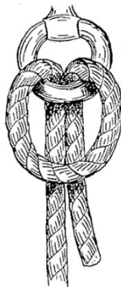
FIG. 31.—Lark's head with toggle (*A*) withdrawn.
