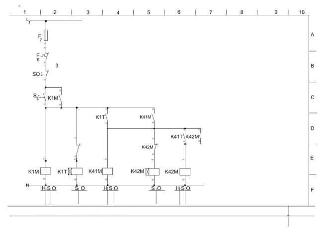
Plan of commissioning command circuit electromotor Cage Rotor three-phase 2 resistors starters 4kw and up, Statoric resistors
