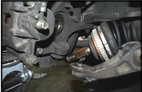
This trick basically allows a 1/2" ratchet's handle to rest in between both metal suspension components and separate the two without damaging the rubber ball joints. An alternative is to use a pickle fork which may tear at the grease ball joints if done improperly. If you have access to a ball joint separator, then I *recommend* using it as this is the proper method for ball joint separation.
