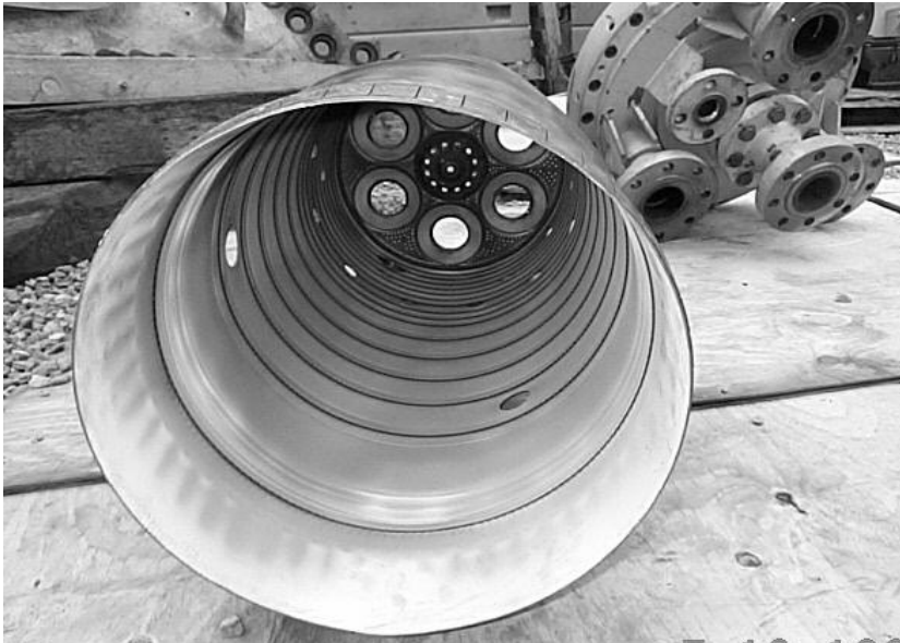
Fig. 2.1. A Combustion Chamber Can. [From Shepherd, D.G., Introduction to the Gas Turbine, D. Van Nostrand Co., Inc.
