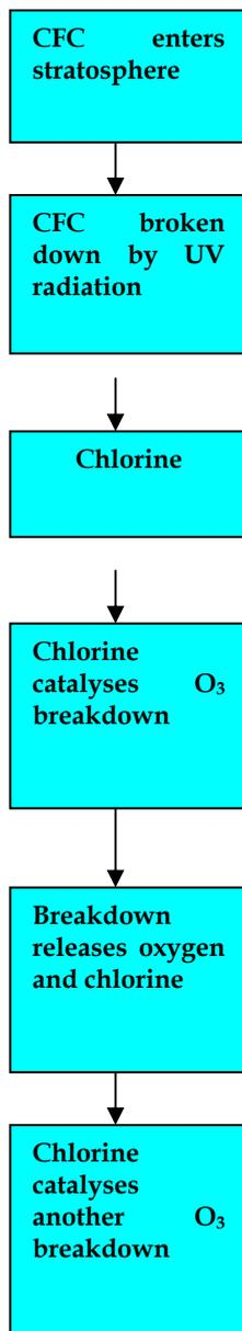
Fig. 7. The process of ozone depletion (Trevor, 2007)
