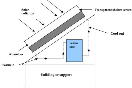
Fig. 1. Solar heater for hot water
