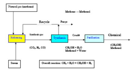
Fig. 5. Schematic process flowsheet
