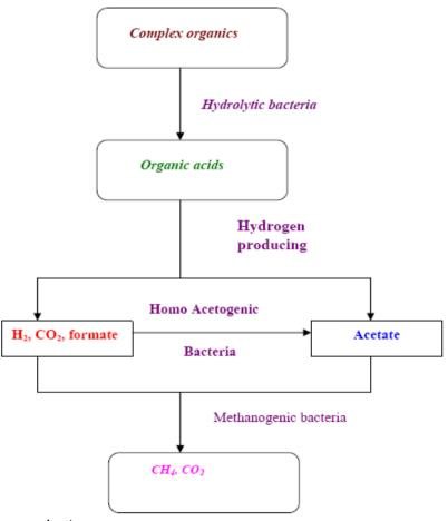
Fig. 3. Biogas production process
