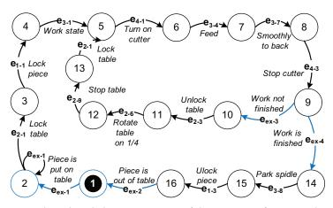
Fig. 13. The required machine behaviour in terms of directive specifications. The semantics is as follows:  $e_{ex-1}$  – a workpiece is on the table,  $e_{ex-2}$  – a workpiece is removed from the table,  $e_{ex-3}$  – processing is not over,  $e_{ex-4}$  – processing is over (other events semantics was given here above in the mechanisms description).
