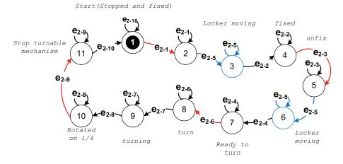
Fig. 9. G<sup>2</sup> CFM – a model of "Turntable" mechanism
