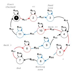
Fig. 10. G<sup>3</sup> CFM - a model of "Spindle" mechanism
