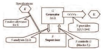
Fig. 3. Interrelationship of supervisory control components in DES
