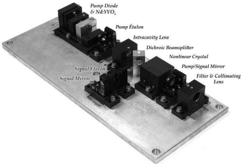
Fig. 3. A well-engineered, all solid-state miniaturised cw-ICOPO. This device consumes just  $\sim 10$ W electrical power, can deliver  $>500$ mW in the down-converted optical fields and requires no forced cooling. The function of the various components is discussed later in the text.
