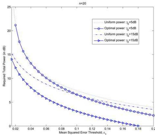
Fig. 5. Optimal power allocation scheme vs. uniform power allocation scheme: The required optimal power to achieve a given MSE of  $\epsilon_1$  as given in (18) is shown in the figure parameterized by local SNR  $\gamma_0$  for  $n=20$  is shown. The comparison of the required uniform power to achieve the same MSE threshold is illustrated.
