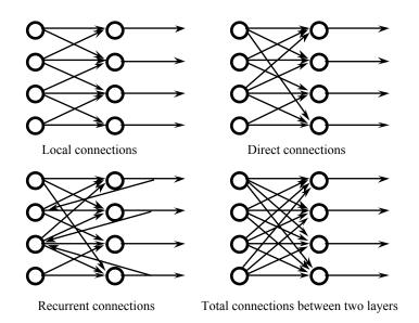
Figure 7. Some models of network connections
