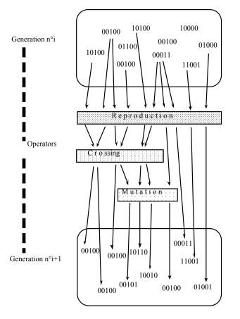
Figure 4. Diagramatic representation of the simple G.A.
