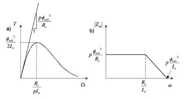
Fig. 4. a) Static characteristic of an axial-symmetric induction machine b) Representation of its mechanical impedance (magnitude in logarithmic scales).
