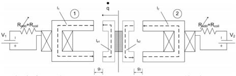
Fig. 7. Sketch of a two electromagnet Semi Active Magnetic Damper (the elastic support is omitted).
