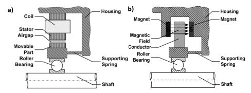
Fig. 2. Sketch of a transformer (a) and a motional damper (b).
