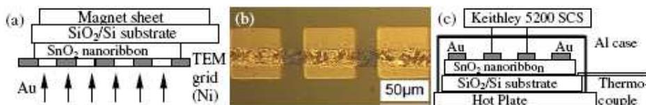
Fig. 2. Deposition of Au contacts along a single SnO<sub>2</sub> ribbon using TEM grids as masks: (a) schematics, (b) optical micrograph of resulting sample, (c), schematics of the testing system.
