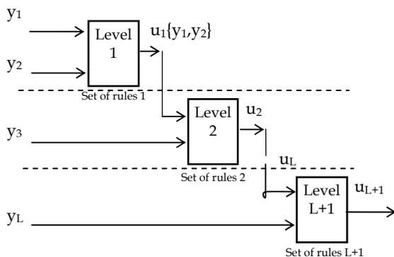
Fig. 2. Schematic representation of a hierarchical fuzzy controller.
