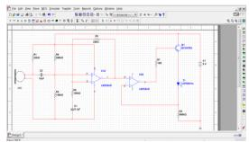
Fig. 2 Transmitter schematic in N.I. Multisim 11.0
