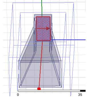
Fig 10 : Figure showing the direction of excitation for a solution frequency of 16Ghz
