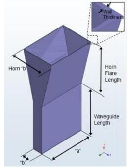
Fig 3 : Structure of the proposed E-Plane Horn Antenna
