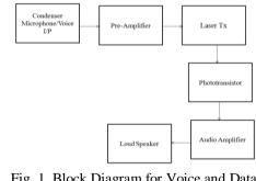
Fig. 1 Block Diagram for Voice and Data Transmission
