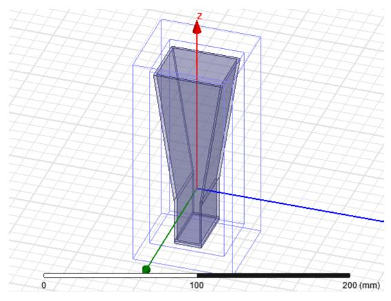
Fig 4 : 3D View of the E-Plane Horn antenna in HFSS for a solution frequency of 8Ghz
