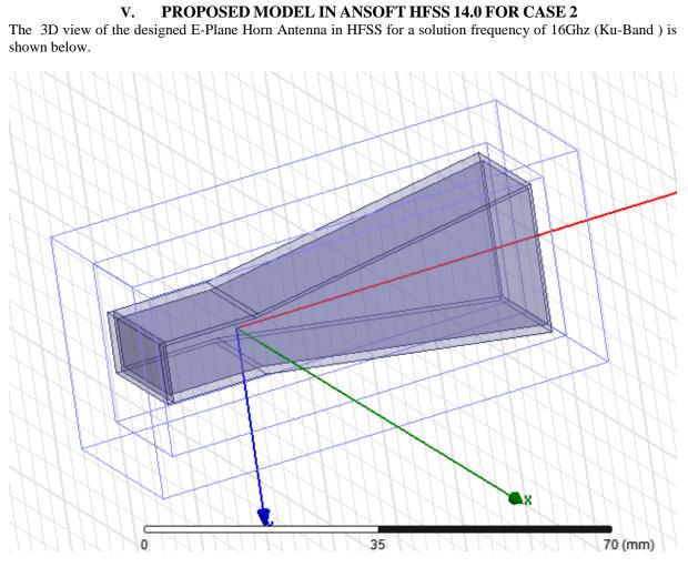
Fig 9 : 3D View of the E-Plane Horn antenna in HFSS for a solution frequency of 16Ghz
