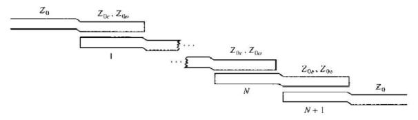
Figure 1. : Layout of an (N + 1)-section coupled line bandpass filter.
