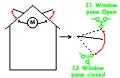
During the day, the window panes open to ventilate the structure from 12:00 to 15:00, at the time of day when, in principle, the temperature is the highest. However, if the temperature is less than 10°C, the window panes do not open, or when they are already open, they close.
