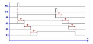
An "On" (**MA**) button authorizes the activation of the first heating element (**S1**). After a time-delay T, the second element (**S2**) starts up. After the same time-delay, the third elements starts up (**S3**), then the fourth element (**S4**) again after time-delay T. An "Off" (**AR**) button deactivates **S1**. The three other elements are progressively deactivated after time-delay T with each deactivation of the preceding element.
