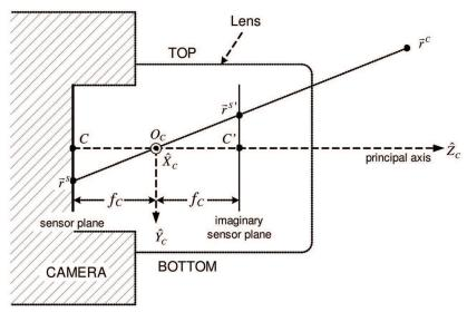
Fig. 1. Right side view of the camera-lens system
