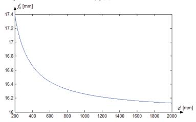
Fig. 4. Camera constant  $f_c$  in terms of the distance d
