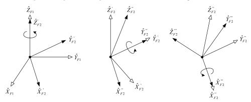
Fig. 5. Representation of the rotations in terms of the ZYX Euler angles
