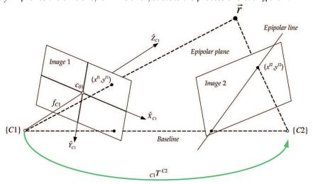
Fig. 7. Stereo-image configuration with epipolar geometry
