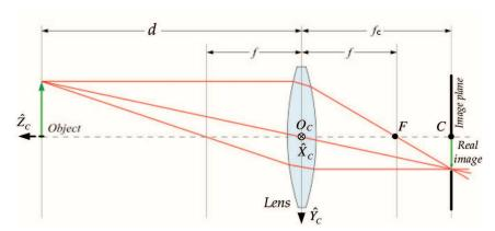
Fig. 3. Left side view of the camera-lens system
