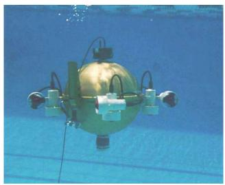
Fig. 11. Omni-Directional Intelligent Navigator (ODIN) vehicle.
