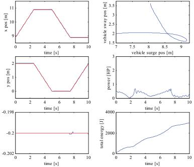
time [s] time [s] Fig. 9. Task-space trajectories (left column), and surge-sway motion, power requirement and energy consumption (right column) for Dynamics-Based planning method for Case II (total decomposition).
