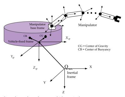
Fig. 1. Coordinate frames for underwater vehicle-manipulator system.
