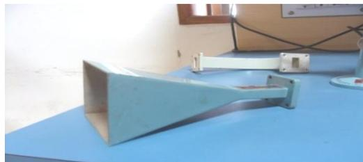
Fig 1 : A Practical Horn Antenna
