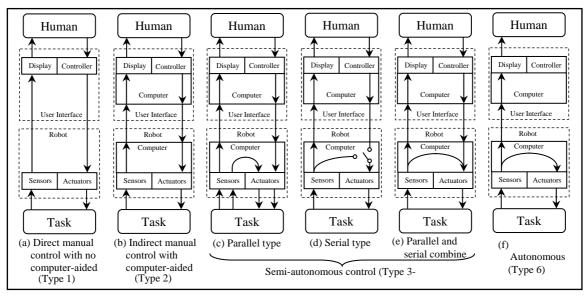
Figure 1. A spectrum of control modes ((Fig. (a), (b), (e) & (f) are adapted and modified from Sheridan (1992) and (Fig. (c) & (d)) are adapted and modified from Yasuyoshi et al. (1993))
