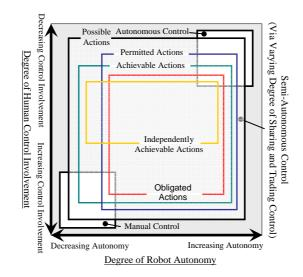
Figure 3. Control modes based on robot autonomy and human control involvement in accordance with varying nested ranges of action of robot
