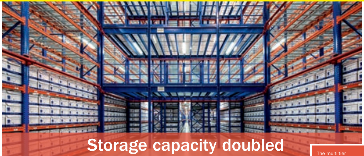
The multi-tier mezzanine system can store up to one million cartons.
