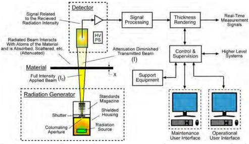
Fig. 2.1 – Diagram illustrating the primary concepts and components associated with transmission-based radiation attenuation gauging.
