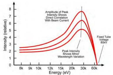
Fig. 3.10 –Illustration of the Bremsstrahlung spectra behavior due to variations in the applied beam current, while maintaining a constant tube potential.
