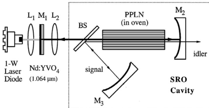
Fig. 6. A simple cw PPLN-Nd:YVO<sub>4</sub> ICOPO (Stothard, Ebrahimzadeh et al. 1998)
