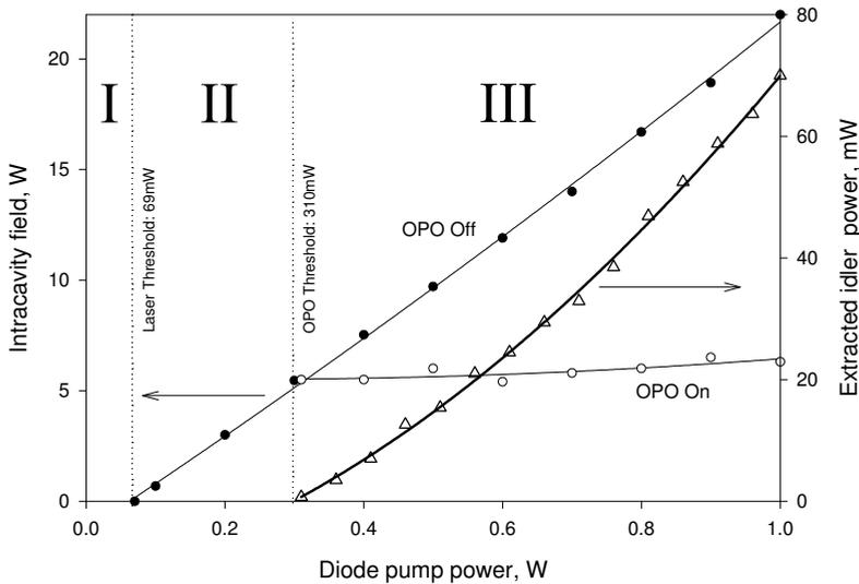
Fig. 10. Extracted idler (triangles) and pump-field with (open circles) and without (closed circles) operation of the OPO as primary diode pump power is varied. The idler wavelength was 3.66 $\mu$ m.
