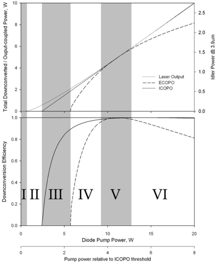
Fig. 4. Down-conversion characteristics of IC- and EC-OPOs
