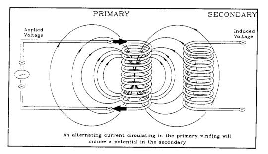
Figure 2-2. Transformer flux lines.
