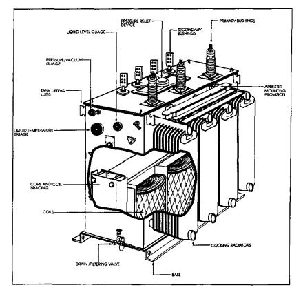
Figure 1-1. Typical power transformer.
