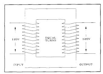
Figure 2-3. Transformer equal turns ratio.
