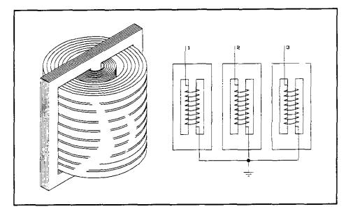
Figure 2-7. Transformer shell construction.
