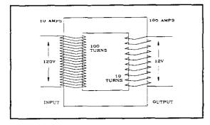
Figure 2-4. Transformer 10:1 turns ratio.
