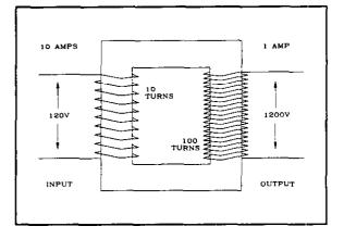
Figure 2-5. Transformer 1:10 turns ratio.
