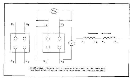
Figure 3-5. Transformer subtractive polarity test.
