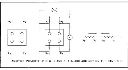
Figure 3-6. Transformer additive polarity test.
