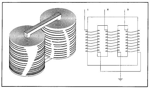
Figure 2-6. Transformer shell construction.
