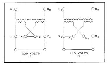
Figure 3-2. Single phase transformer secondary winding arrangements.
