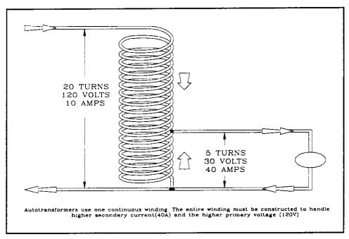
Figure 3-7. Autotransformer.
