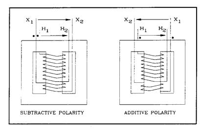
Figure 3-3. Physical transformer polarity.
