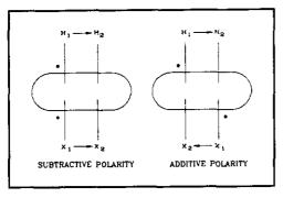
Figure 3-4. Diagrammatic transformer polarity.
