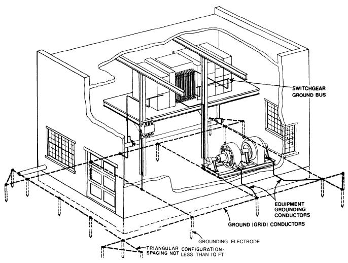
Figure 2-3. Typical grounding system for a building.
