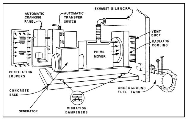
Figure 2-1. Typical installation of an emergency power plant.
