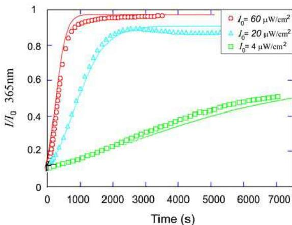
Fig. 10. The effect of photo-bleaching for samples with high dye concentration ( $x/D = 2.2$ ). Three values of irradiation intensity are labelled on the plot. Solid lines are fits to the data with only one free parameter  $\alpha$ , giving  $\alpha = 60$  for the highest intensity,  $\alpha = 20$  for the middle intensity, and  $\alpha = 4$  for the lowest intensity. [Serra & Terentjev 2008b]
