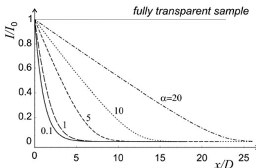
Fig. 7. Transmitted intensity ratio  $I/I_0$  in the photostationary state as a function of the parameter  $x/D$  (proportional to sample thickness or inversely proportional to chromophore concentration) for several values of  $\alpha$ . At small  $\alpha$  the decay is exponential; the light penetrates deeper into the sample as  $\alpha$  increases, as the decay tends to be linear. [Serra & Terentjev 2008b]
