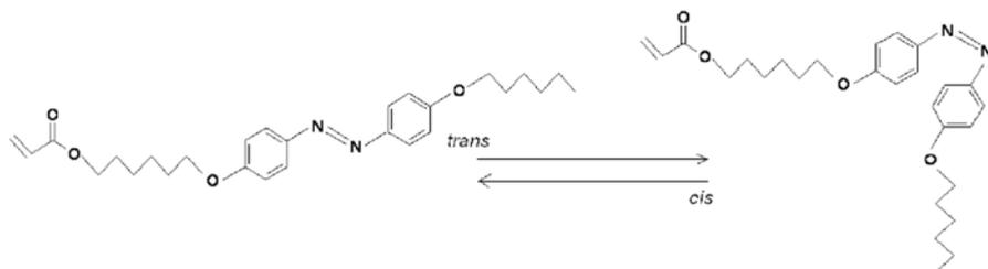
Fig. 3. The monomer used AC<sub>6</sub>AzoC<sub>6</sub> has an acrylate head group followed by a carbon chain where the azo-group is attached. It is schematised here in its two isomers, *trans* and *cis*.
