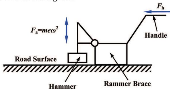
Fig. 5 the mechanism of the inertia rammer
