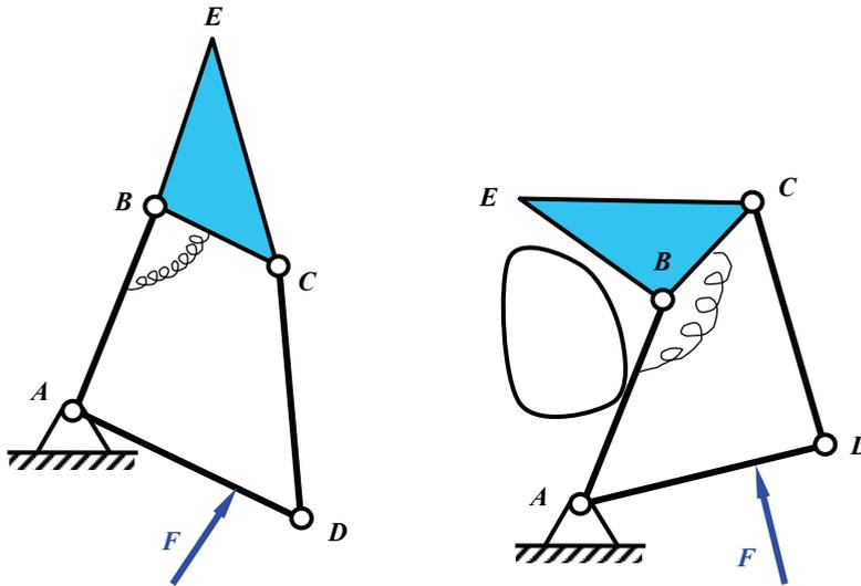
Fig. 8 underactuated mechanical finger with return actuation
