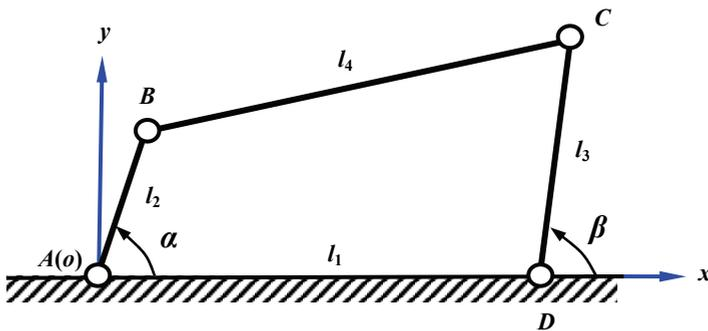
Fig. 7 a planar four-bar mechanism with two actuations
