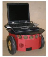
Figure 9. The Pioneer 3-DX robot with a laptop computer
