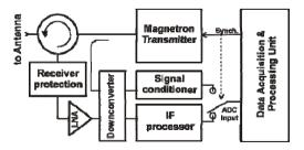
Fig. 5. Typical block-diagram of magnetron based radar.
