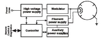
Fig. 6. Block-diagram of magnetron transmitter.
