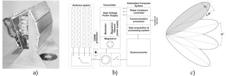
Fig. 4. Outline (a), block diagram (b), and antenna pattern (c) of Ka band airborne scanning radar.
