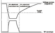
Fig. 7. Waveforms of voltage pulse across magnetron and RF envelope.
