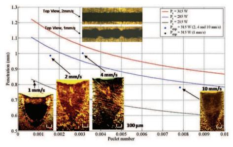
Fig. 5. Model validation for low speed welding of AA 7075-T6
