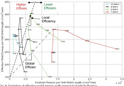
Fig. 8. Variation of effective weld energy with respect to keyhole fluence
