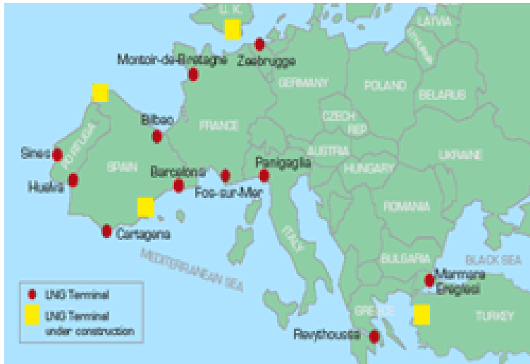
Fig. 2. Europe: Regasification Terminals for LNG Imports Source: Energy Information Administration (EIA), The Global Liquefied Natural Gas Market
