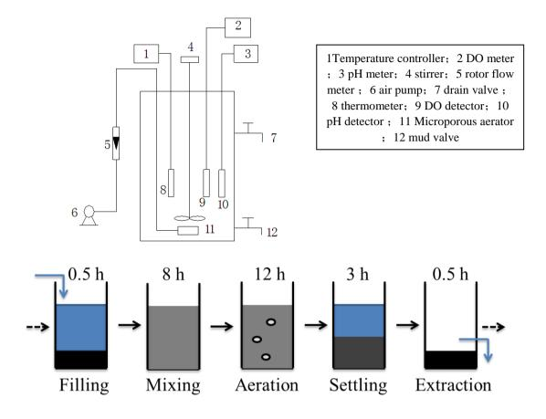
Figure.2 Schematic diagram of SBR reactor
