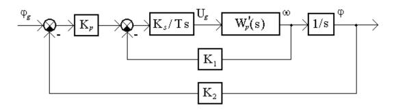
Figure 3. Structure of the position control system loop for the manipulator shoulder unit
