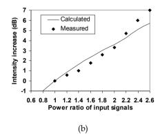
Fig. 3. Theoretical phase difference (a) and intensity increase (b) of the output signals for the unbalanced configuration from the balanced configuration verses power ratio of the two detector input signals, respectively. The experimental results are shown as the points.
