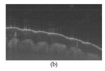
Fig. 6. *In vivo* images of human finger tip acquired by our full range swept-source optical coherence tomography using the 3x3 Mach-Zehnder interferometer with unbalanced differential detection technique. (a): the image was generated using only a single detector. (b): the complex signals were used.
