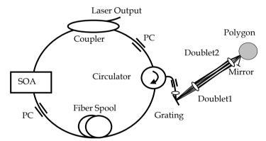
Fig. 7. Schematic diagram of a FDML wavelength-swept laser shown with a ZEMAX ray-tracing of the polygon-based narrow-band filter.
