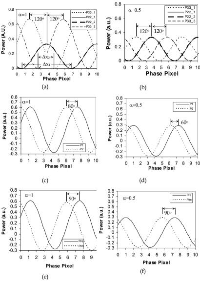
Fig. 2. Theoretical waveforms before (a, b) and after (c, d) the differential detection and after the quadrature signal calculations (e, f) when the attenuation  $\alpha$  = 1 (a, c, e) and 0.5 (b, d, f), where  $\alpha$  = 1.0 and 0.5 correspond to the unbalanced by a factor of 2 and balanced configurations, respectively.
