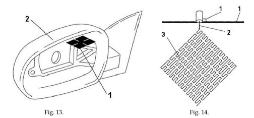
In the Figure 14 is shown another example of space-filling antenna, based of a fractal curve, for AM/FM reception. The antenna is fed as a monopole and is placed inside a rear view mirror support.
