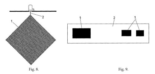
Both conducting sheet (1) and counterpoise are connected through a conducting strip. Each conducting sheet is fed by a separate pin.
