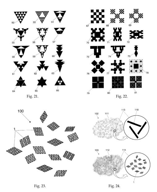
Figure 24 shows a comparison between a conventional chaff cloud with regard to a fractal or multilevel structure chaff cloud. Conventional chaff is formed substantially by linear or straight strip dispersers of a length determined by the wavelength of the radar. The fractal chaff are smaller for the same operating frequency, therefore a fractal chaff cloud can be made denser than a conventional one, providing a larger radar cross-section (RCS) and remaining floating in the air for a long time.
