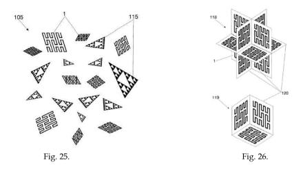
Figure 25 shows a mix of multilevel and fractal structures with diverse sizes forming a radar cloud. The sizes and geometries of the structures can be made to design the frequency signature for the whole chaff cloud.
