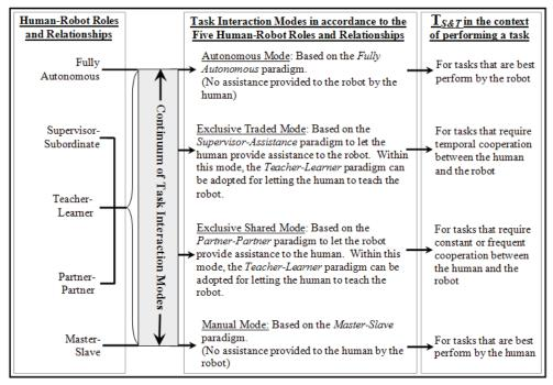
Figure 3. Range of task interaction modes in accordance to the characterisation of  $T_{S \otimes T}$  in different human-robot roles and relationships depicted in Fig. 2
