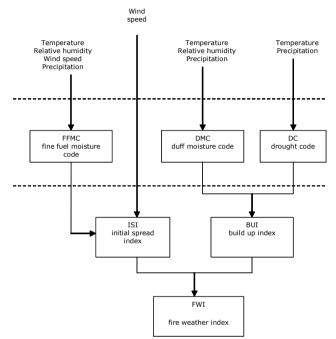
Fig. 3. Canadian Fire Weather Index (FWI) System components (adapted from Van Wagner, 1987).
