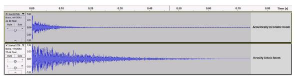
Figure 2.1: Echoes of the impulse can especially be seen in the echoic room, where the signal takes longer to decay.
