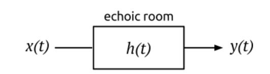
Figure 3.1: Block diagram of the echoic room as an LTI system with impulse response h(t) where y(t) is the echoed version of the input x(t).
