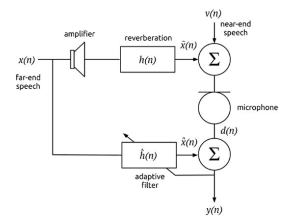
Figure 1.1: Block diagram example of typical acoustic echo cancellation.
