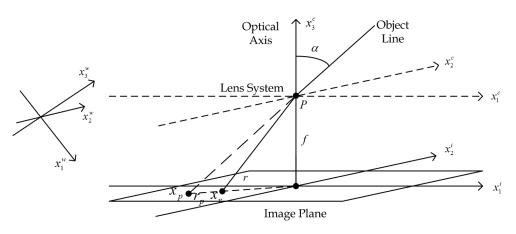
Fig. 2. Illustration of the CCM with the world, camera and image coordinate systems. Two points in the image are defined, one undistorted,  $x_p$ , and one radially distorted,  $x_r$ .
