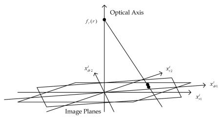
Fig. 4. The leaning image compensation converts between leaning and non-leaning detectors so that a line between the points on the two planes hits the optical axis at a point  $f_i(r)$  units from the principal point.
