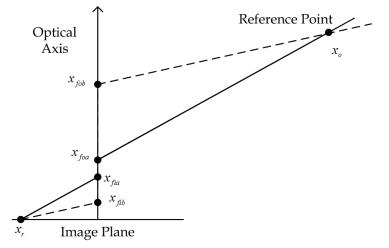
Fig. 7. If the distance to the reference does not vary two different sets of camera parameters *a* and *b* can both give a small error norm in both image and object space. The calibration can not determine if situation *a* or the dotted *b* in the figure is the right one.
