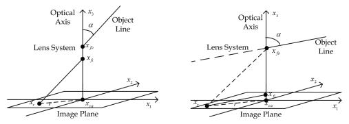
Fig. 3. Geometrical construction of the GCM, with different inclination angles. The points  $x_{f_i}$  and  $x_{f_i}$  can slide along the optical axis depending on r, the distance to the centre
