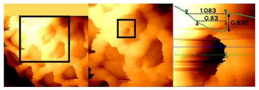
Fig. 3. Inset represents the AFM image of hole after being perforated at 0.5 mW fs-laser pulse. The extrusion of any cytoplasmic contents out of the pollen grains was not observed at the said fluence.
