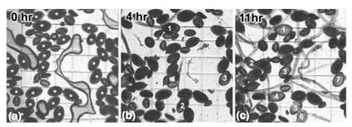
Fig. 4. Sequential images of pollen tube growth before (a) and after fs-laser treatment (b-c). fs-laser beam was focused into the interior of the wall inside pollen ornament. The pollens marked with asterisks were irradiated with laser beam with the fluence of 8  $\mu$ J/pulse. Seven pollens out of 26 treated pollens in this run were eventually geminated to grow the pollen tube.
