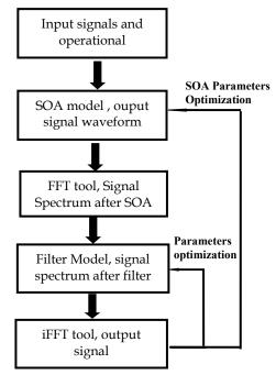
Fig. 2. Analytical process for all-optical signal processing schemes with fixed configurations
