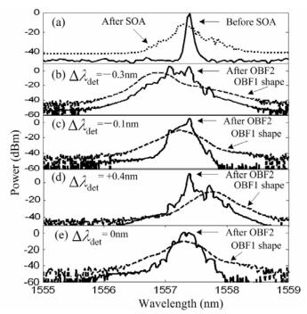
Fig. 8. Spectra of converted signal with different detuning, (a) the probe spectrum before and after SOA, (b)-(e) are the output spectra of converted signal when the OBF1 detuning is -0.3nm, -0.1nm, +0.4nm, and 0nm, respectively.
