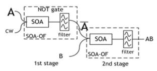
Fig. 14. Schematic diagram for all-optical logic AND gate with cascaded SOAs
