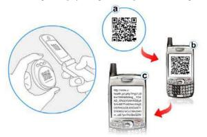
Fig. 9. A procedure for temperature data collection using a wearable sensor and a mobile phone. (a) A QR code image. (b) A QR code captured by a camera built into a mobile phone. (c) Original data recovered from the image captured by a mobile phone (QOL Co. Ltd., 2008).
