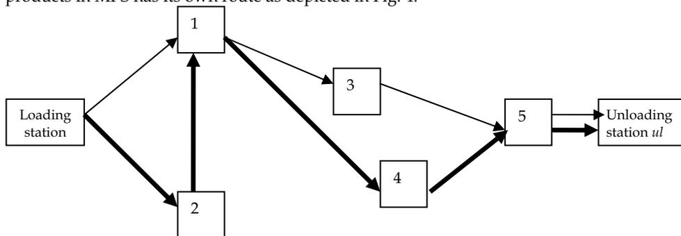
Fig. 4. An example of a simple technological network with two linear product routes and five processing machines, depicted by the squares, where  $\longrightarrow$  denotes the route for product  $a$ , and  $\longrightarrow$  denotes the route for product  $b$  (from Kats et al. (2007))
