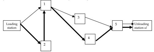
Fig. 4. An example of a simple technological network with two linear product routes and five processing machines, depicted by the squares, where  $\longrightarrow$  denotes the route for product *a*, and  $\longrightarrow$  denotes the route for product *b* (from Kats et al. (2007))
