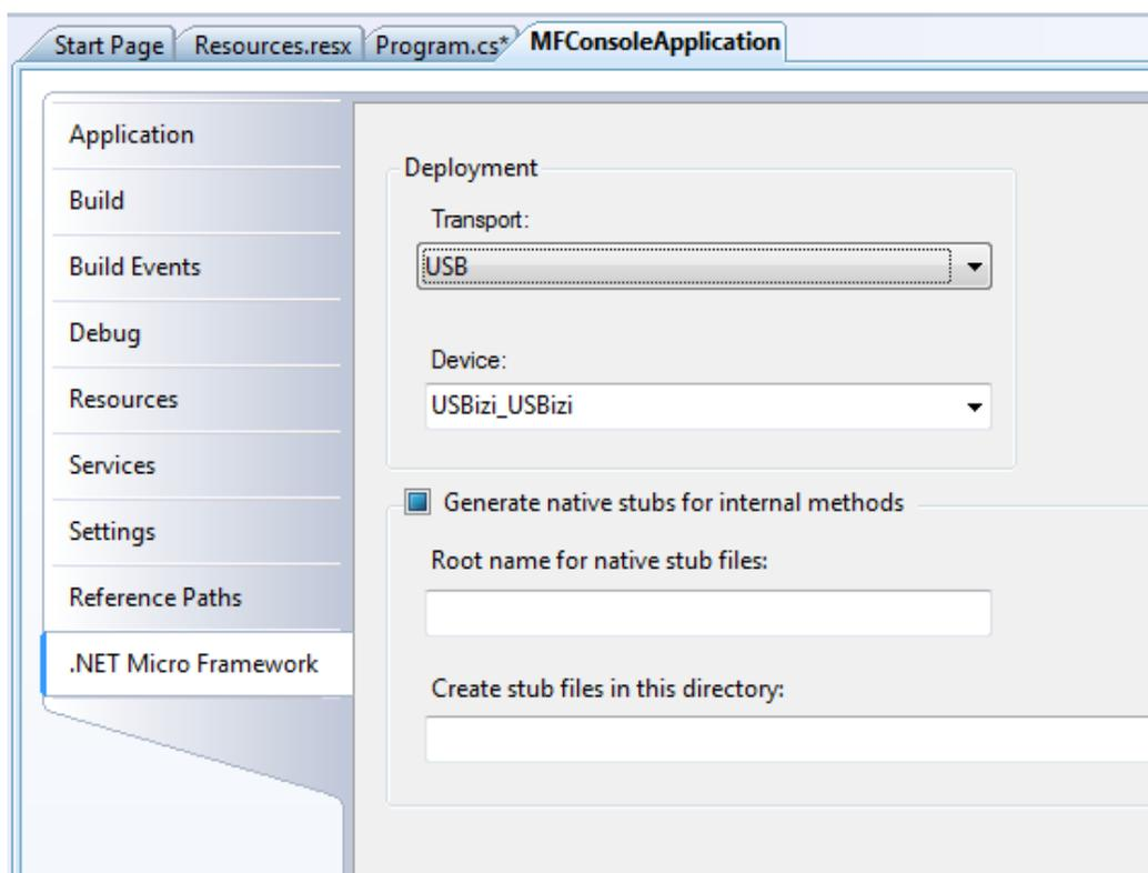
Pressing F5 will now send our simple application to FEZ and it will run right inside the real hardware. Switching from emulator to real hardware is that simple!
