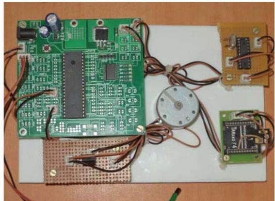
Figure 15. The D.C. Motor Module
