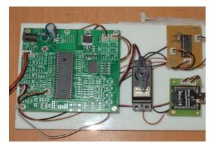
Figure 12. The Servo Motor Module
