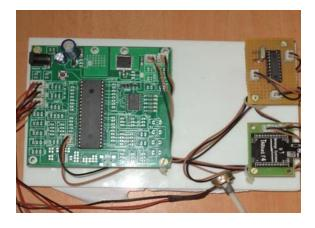
Figure 13. The Engine Control Module
