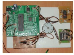
Figure 15. The D.C. Motor Module
