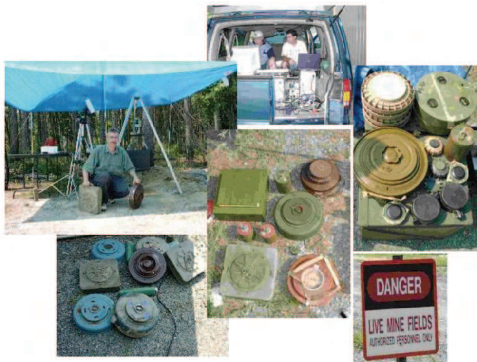
Fig. 2. Collection of live mines and experimental setup for dynamic impedance measurements of mines at U.S.Army testing ground
