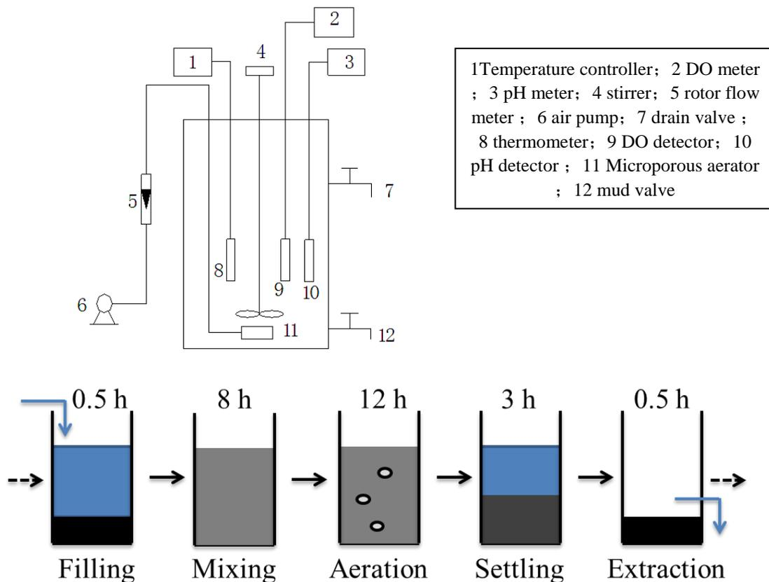
Figure.2 Schematic diagram of SBR reactor
